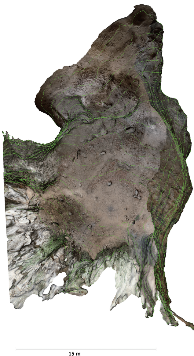
Fig. 9 The present Teshik Tash Cave plan documented through a photogrammetric survey. Contour: 50 cm intervals.
