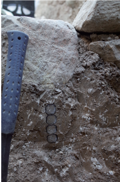
Fig. 3.3 Virgin soil underneath the building stones, with plastic cubes for anisotropy of magnetic susceptibility measurement
