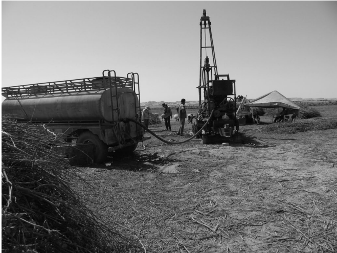
Fig. 2 The boring machine (centre) and the water tank (left) at the locality RQ-1.
