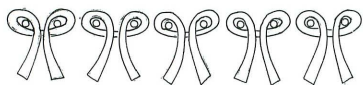
Fig. 1 Style A structure of pile weave: "Ghiordes knot" seen on Specimens i to v
